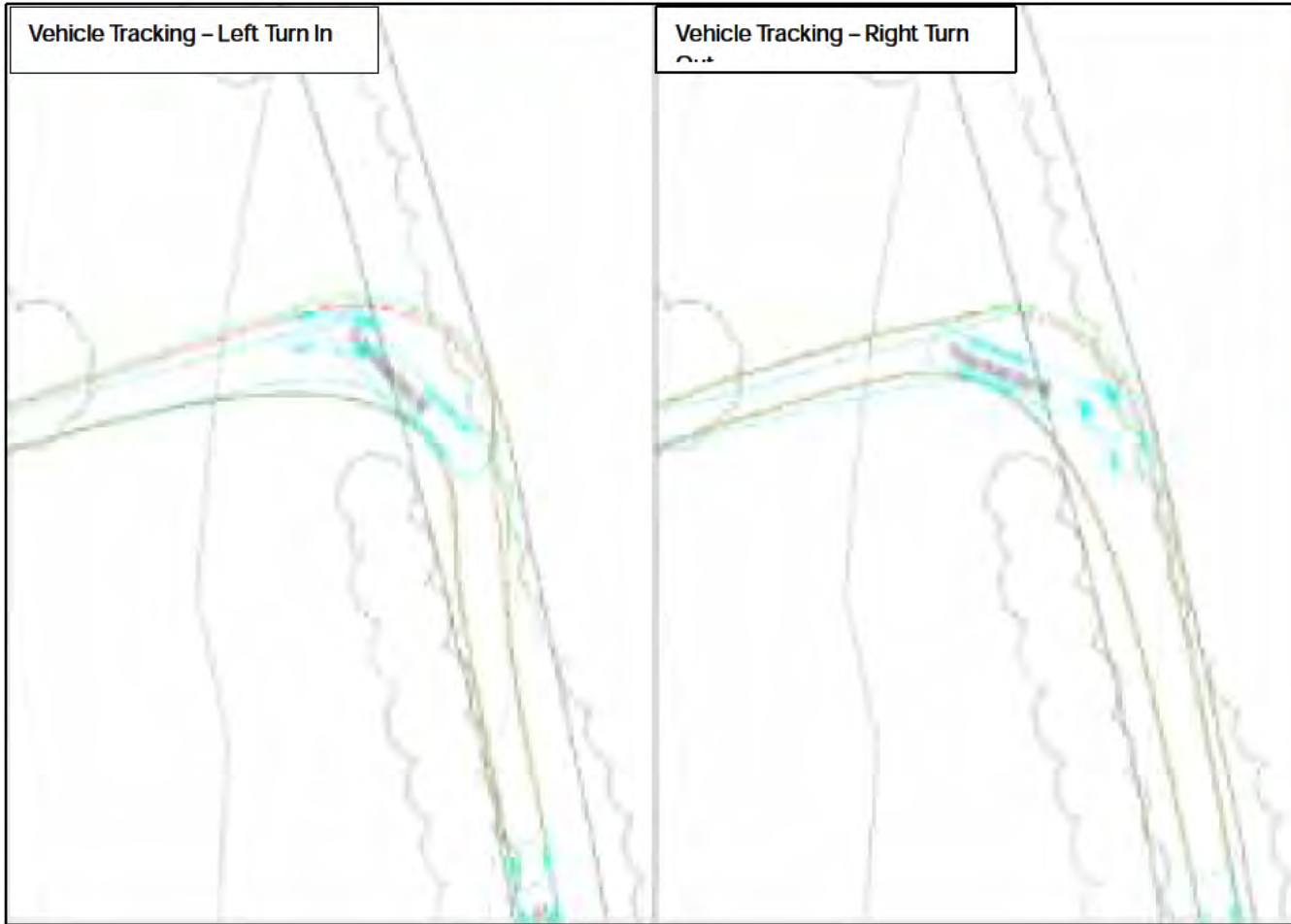
Figure 12: Sunnica East – Access D – Vehicle Tracking
