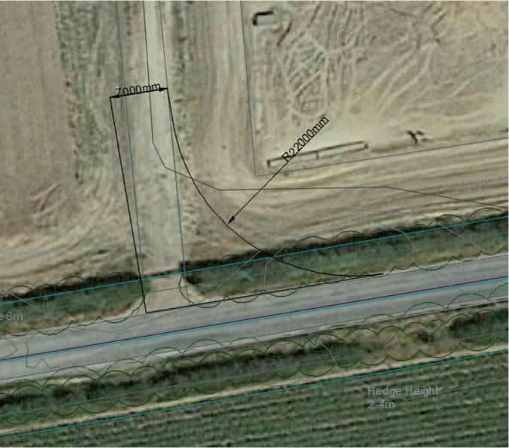
Figure 16: Crane Entry Option 2 – Junction Works Area
