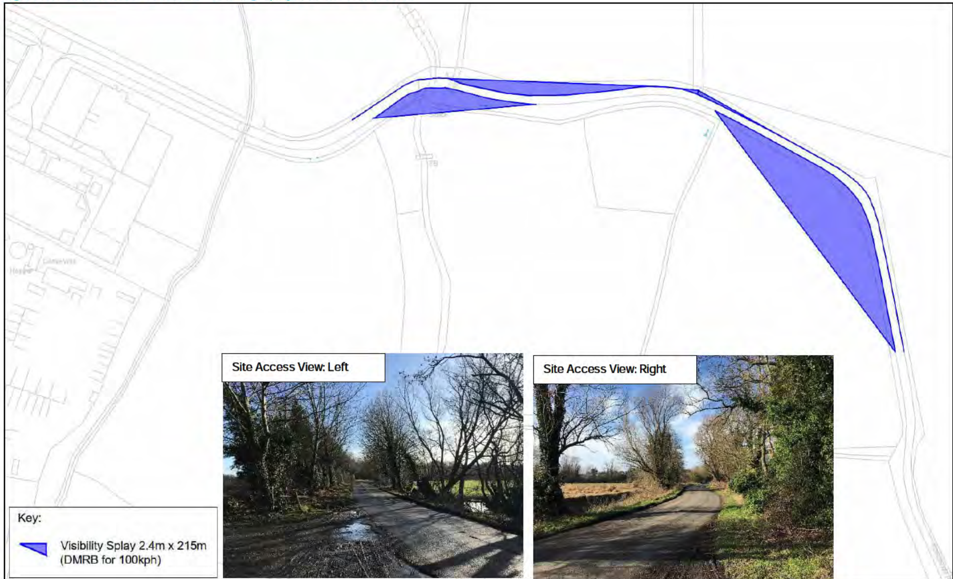
Figure 37: Sunnica West- Access D – Visibility Splay and Site Visit Photos
