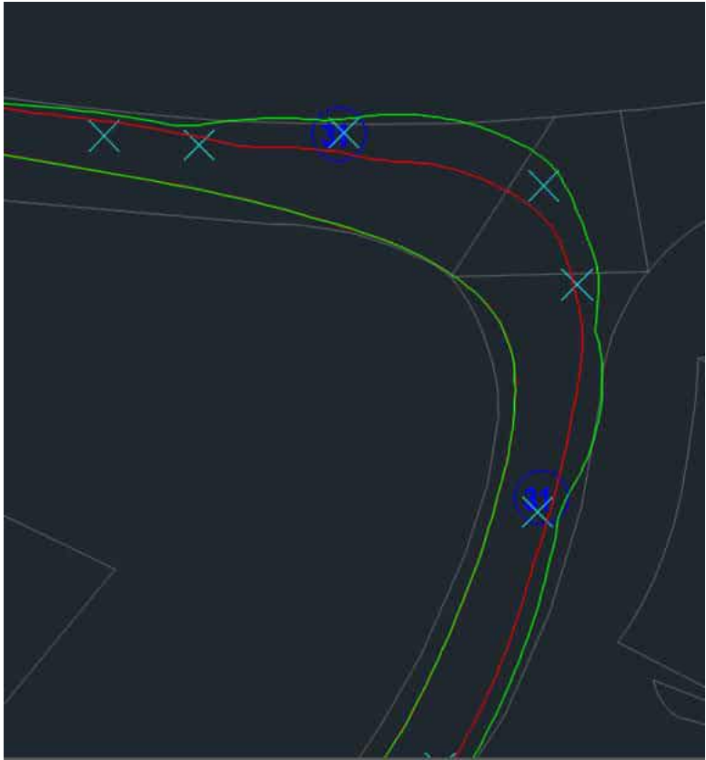
Figure 48: Swept Path Analysis: 400T Crane A11/Elms Road
