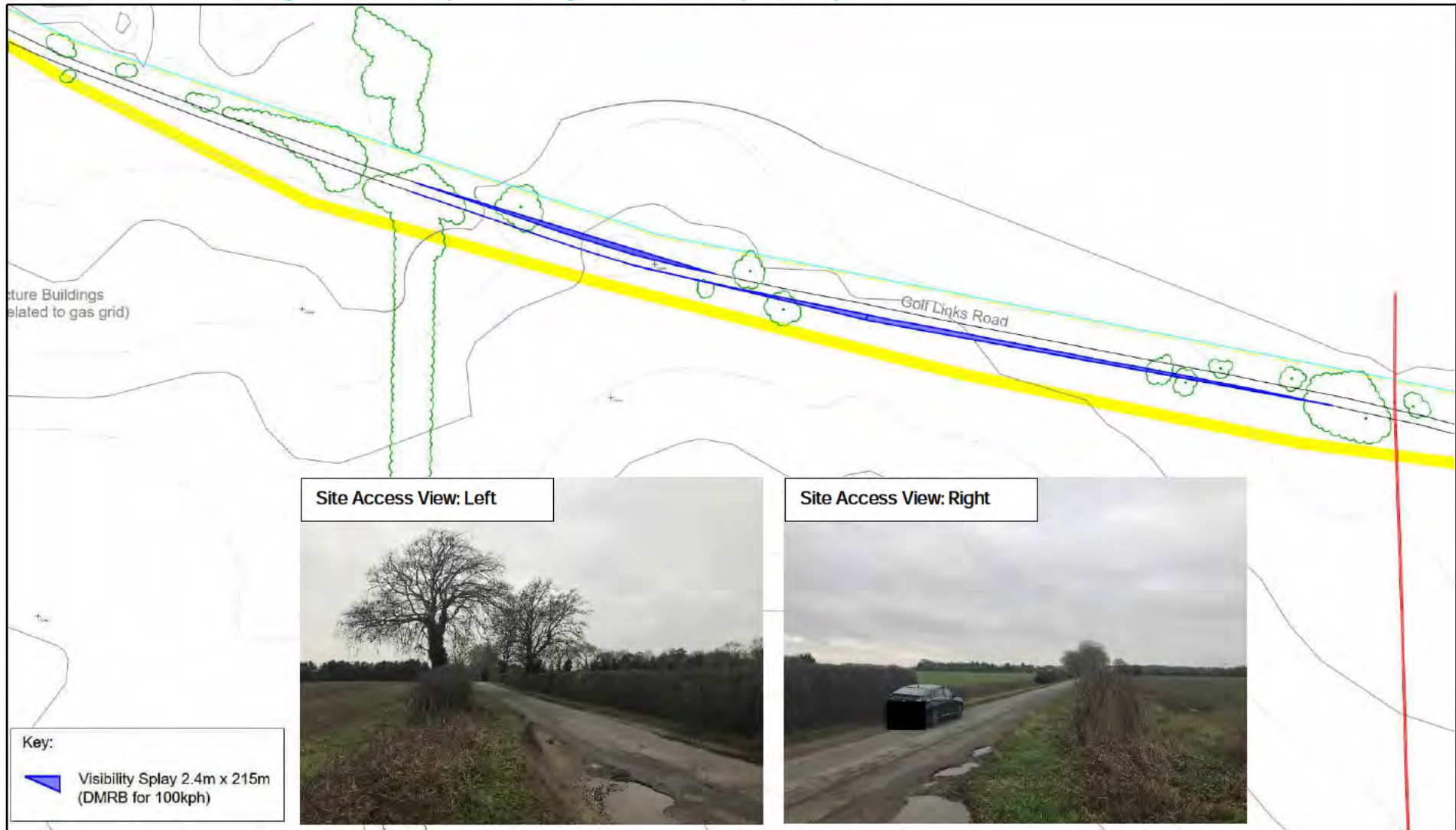
Figure 22: Sunnica East – Access I – Visibility Splay and Site Visit Photos Site access not to be used during the construction phase and only to be used in the operational phase
