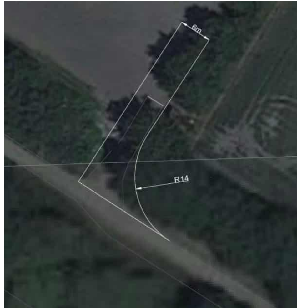
Figure 3: Option 2 – Indicative Junction Works Area
