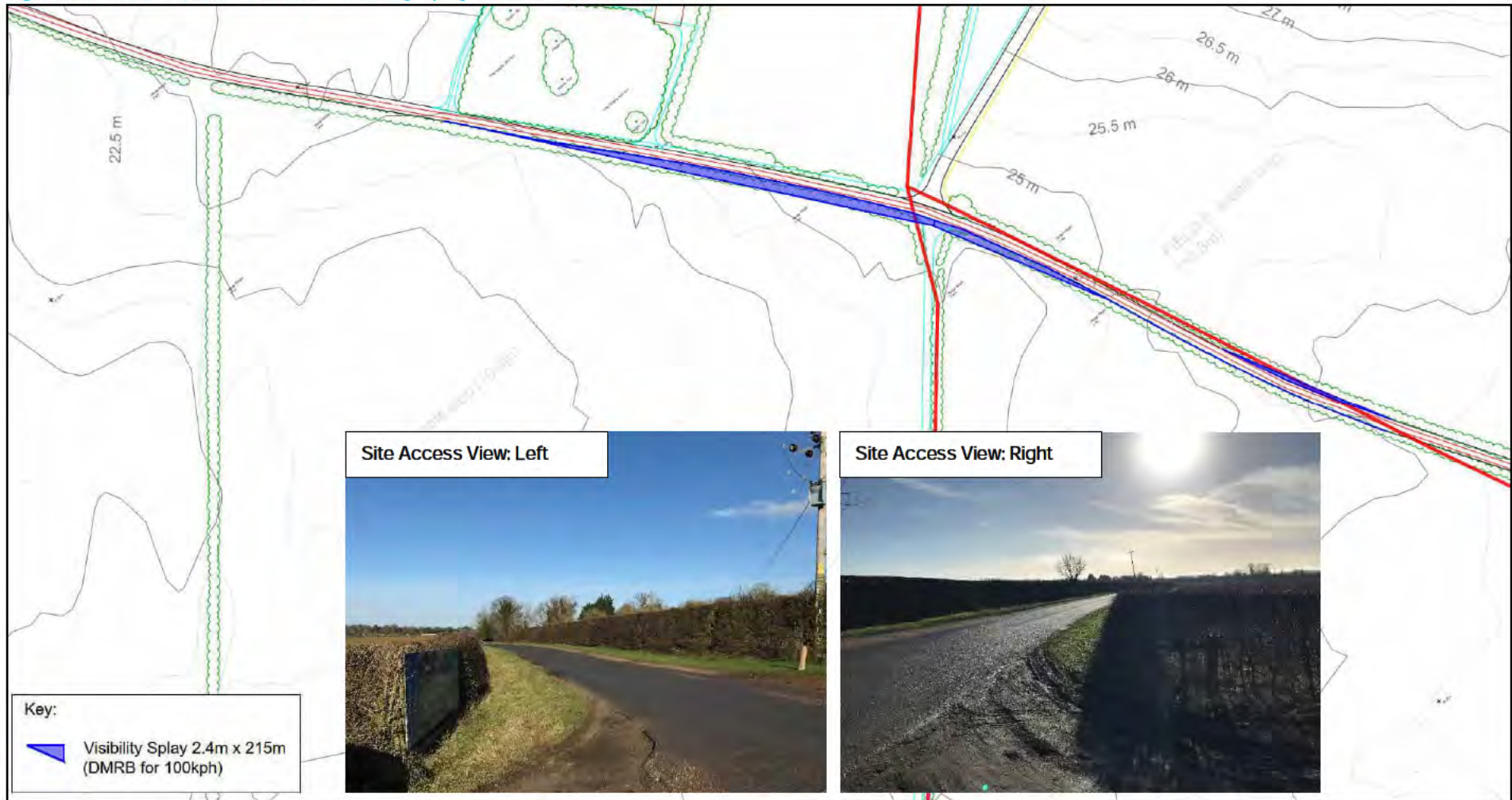
Figure 25: Sunnica West- Access A - Visibility Splay and Site Visit Photos
