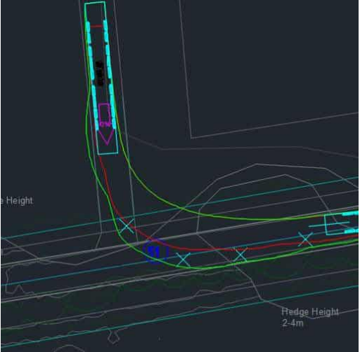
Figure 11: 1000T Crane Egress
